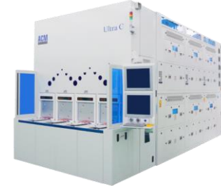
Single High Temp SPM Cleaning for metal removal and PR Strip at advance node
